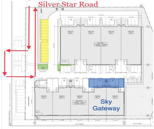
The red arrows show the flow in and out using the new gravel loop.
